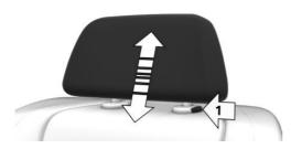
The height of the head restraints can be adjusted.
