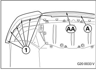
Secure the Pro carbon front attachment **AA** with the expanding rivets (1).
