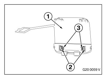
Remove the cover on the towing eyelet cover (1). Carefully bend the two barbs (2) on the rear of the towing eyelet cover (1) towards the inside without deforming the holders (3) too badly, and press them out towards the front of the towing eyelet cover (1).
