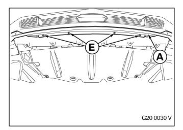
Check the accurate fit on the wheel arches again, secure it with adhesive tape and secure the black front attachment **A** from below using the screws **E**.
