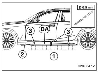
Drill the 14 holes (1) from the side sill add-on section **DA** with a diameter of **6.5 mm** in the side sill (2). Remove the adhesive tape (3) and the side sill add-on section **DA**.
