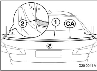
Position the carbon rear spoiler **CA** on the boot lid (1), centre it and mark the position (2) with suitable tools.
