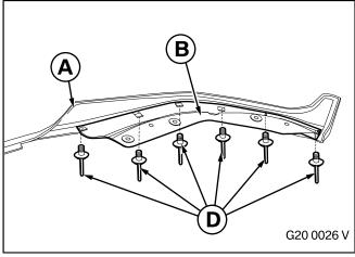
Rivet the front attachment support  ${\bf B}$  to the black front attachment  ${\bf A}$  from below using the expanding rivets  ${\bf D}$ .
