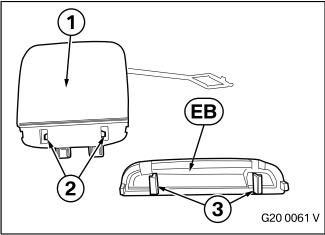
The body-coloured towing eyelet cover (1) will be reused.
