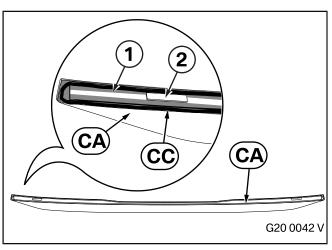
Abrade and clean the edge area (1) of the carbon rear spoiler **CA** using suitable products.
