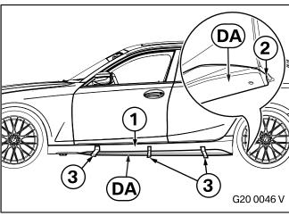
Position the side sill add-on section **DA** on the side sill (1). The rear contour (2) of the side sill add-on section **DA** must be flush with the rear contour of the side sill (1). Secure the side sill add-on section **DA** using suitable adhesive tape (3).
