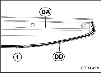
Follow the instructions for use for the liquid adhesive **DD**. Apply the liquid adhesive **DD** to the side sill add-on section **DA** only on the external side of the car at the installation position.
