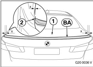
Position the matt black rear spoiler **BA** on the boot lid (1), centre it and mark the position (2) using suitable tools.
