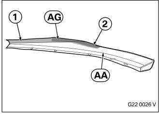
Clean the inner surface (1) of the right front attachment **AA**. Prime the part of the area (2) which comes into contact with the remaining adhesive tape, as shown, with primer **AG**.
