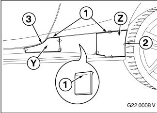
Place the rear template **Z** on the start of the radius (1) and (2) and secure it using suitable adhesive tape.
