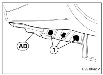
Apply dots of liquid adhesive **AE** to the abraded surfaces (1) of the underbody console **AD**.
