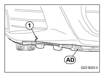
Remove the backing foils (1) on the left and right completely from the underbody console **AD**.
