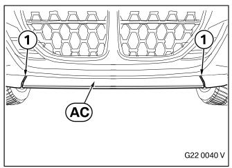
Position the centre front attachment **AC** in the middle between the two side sections so that there is an even gap (1) on both sides.
