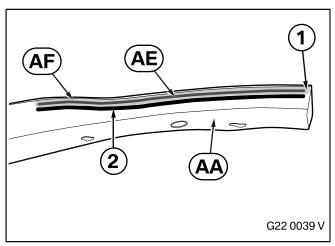
Clean the inner surface (1) of the right front attachment **AA** above the foam strip (2), as shown, with cleaner **AF**.
