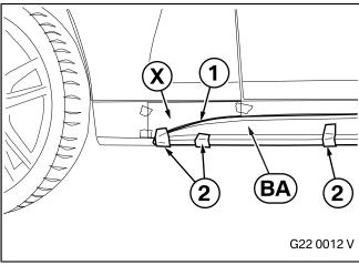
At the same time the carbon side skirt attachment **BA** should be positioned on the front of the car in the contour (1) of the front template X.
