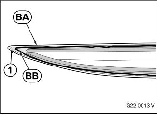
Apply a bead of the liquid adhesive **BB** to the surface (1) all round the carbon side skirt attachment **BA**.
