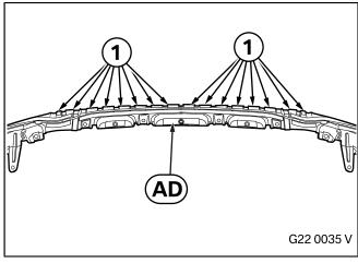
Abrade the surfaces (1) on the top of the underbody console **AD** using suitable tools and clean it with cleaner **AF**.
