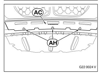
In addition to checking gap, align the centre front attachment **AC** in the x and z directions so that the surfaces of the front attachments align with each other evenly. They must be secured in this position using adhesive tape (1) as shown in the illustration. Use additional to secure the centre front attachment **AC** if necessary.
