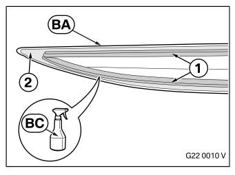
Abrade the surface (2) on the inside of the carbon side skirt attachment **BA** outside the foam tape (1) using suitable tools and then clean it with cleaner **BC**.
