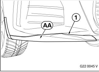
Now check the position to make sure that the top edge (1) of the right front attachment **AA** runs flush with the design edge of the front apron. ◀
