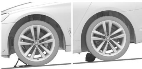
If it is necessary to change a wheel on a slight downhill slope, place chocks and other suitable objects, for example stones, under the wheels of the front and rear axles in the opposite direction to the direction of roll.
