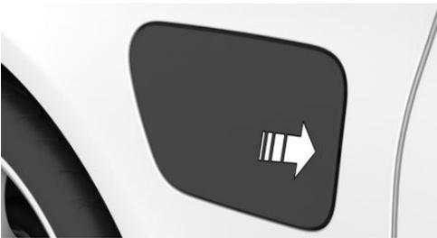
2. Remove cover from charging cable connector if necessary.
