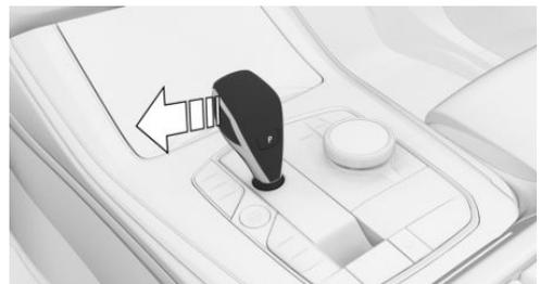
Activate sport programme/manual operation: Press the selector lever out of selector lever position D to the left.
