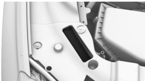
The vehicle identification number is in the engine compartment, on the right-hand side of the vehicle.
