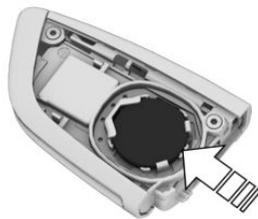
4. Insert a new type CR 2032 battery with the positive side facing upwards.
