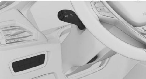
The light switch panel is located next to the steering wheel.
