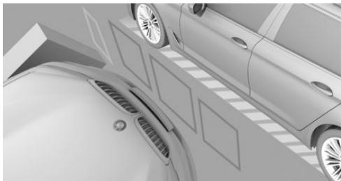
Obstacle markings are displayed at the sides of the vehicle to protect the vehicle's flanks.
