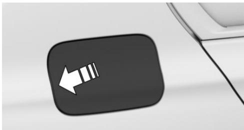
2. Turn the fuel tank cap anticlockwise.
