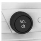
Press and hold the button, until the OFF display on the instrument cluster turns off.
