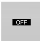
OFF is shown in the instrument cluster. The drive is switched off and standby state switched on.
