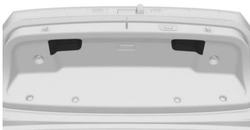
Pull the boot lid down using the handle recess.
