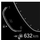
An arrow next to the petrol pump symbol shows which side of the vehicle the fuel filler flap is on.
