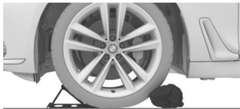
Place chocks or other suitable objects in front of and behind the wheel directly opposite to the one being changed.
