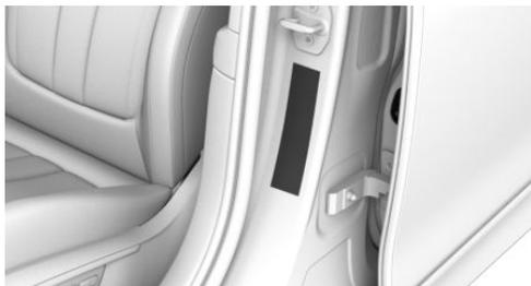
The tyre inflation pressure inscriptions can be found on the tyre pressure plate on the door pillar.
