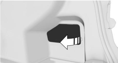
2. Pull the green tag with the fuel pump symbol. Fuel filler flap is unlocked without making any noise.
