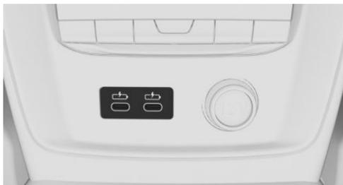
A USB interface with two USB ports is located in the centre console in the rear.
