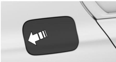
2. Turn the fuel tank cap anticlockwise.
