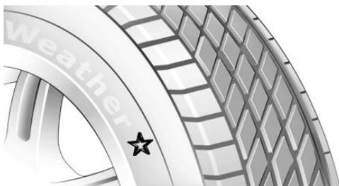
Certain makes of tyre are recommended by the manufacturer of the vehicle for each tyre size. The tyre brands can be identified by a star on the side wall of the tyre.
