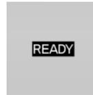
When drive-ready state is switched on, READY is shown in the instrument cluster.
