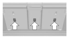
Depending on the equipment fitted in the vehicle, there are two outer mounting points or three other mounting points for child restraints with tether straps.
