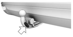
There is an eye on the trailer tow hitch for fastening the trailer securing cable.
