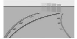
Depending on the equipment, obstacles behind the vehicle are detected by the Park Distance Control PDC sensors.
