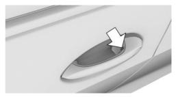
With your finger, touch the grooved area on the handle of a closed vehicle door for approximately 1 second, without gripping the door handle.
