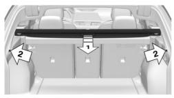
Remove luggage compartment cover, arrow 1, and hang on the brackets on both sides, arrow 2.
