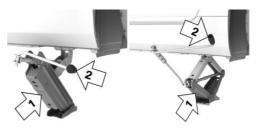
Guide the jack into the rectangular recess of the jacking point closest to the wheel to be changed.
