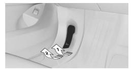
2. After releasing the lever, pull the lever again, arrow 2.
