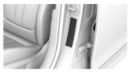
The tyre inflation pressure inscriptions can be found on the tyre pressure plate on the door pillar.
