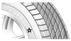
Certain makes of tyre are recommended by the manufacturer of the vehicle for each tyre size. The tyre brands can be identified by a star on the side wall of the tyre.
