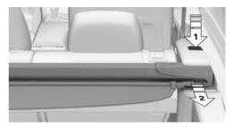
Press the release button, arrow 1, and pull the case for the luggage compartment cover towards the rear, arrow 2.
