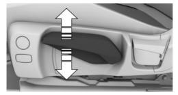
Pull the lever up or press the lever down repeatedly until the seat reaches the desired height.
