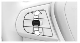
While the system is interrupted, press the rocker switch up or down once. The system is activated.
