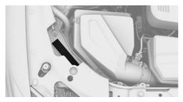
The vehicle identification number is engraved in the engine compartment, on the right-hand side of the vehicle.
