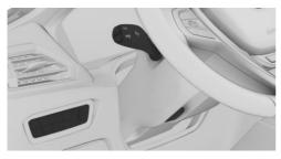
The light switch panel is located next to the steering wheel.
