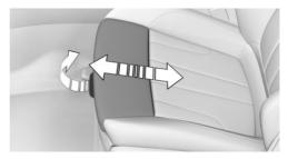
Pull the lever on the front of the seat and adjust the thigh support forwards or backwards.
