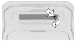
2. To remove it, slide the warning triangle to the side.
