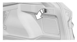
Fold open the bag holder until it detectably engages in the lower position.
