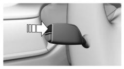
Press the button on the turn indicator lever repeatedly until the desired widget is selected.
