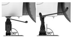
7. Raise by cranking until the jack is supported on the ground with its entire surface and the wheel in question is at most 3 cm, 1.2 inches off the ground.
