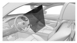
The camera in the roof lining detects gestures made in the area of the centre console at the height of the Control Display.
