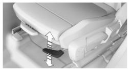
Pull the lever up or press the lever down repeatedly until the seat reaches the desired angle.
