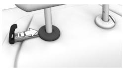
4. Press and hold the integrated key and the button simultaneously, arrows 1, and pull the head restraint fully out.
