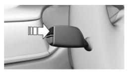
2. Press and hold the button on the turn indicator lever.
