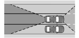
Radar sensors monitor the area adjacent to the vehicle from a minimum speed up to approximately 210 km/h, 130 mph.
