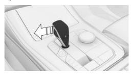
Activate sport programme/manual operation: Press the selector lever out of selector lever position D to the left. Manual operation:
