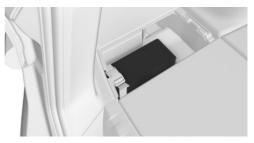
The Mobility System is located in a bag in the left storage compartment of the boot. To remove it, loosen the tensioning strap.
