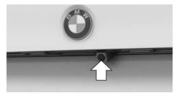
The camera is located in the handle strip of the tailgate.
