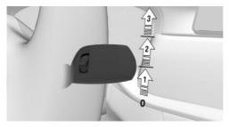
Press the lever upwards to the desired position.
