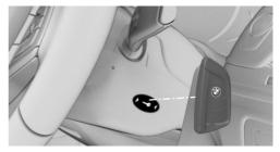
Drive-ready state cannot be switched on if the vehicle key has not been detected.
