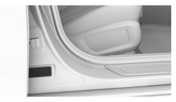
The vehicle identification number is on the type plate on the right-hand side of the vehicle.
