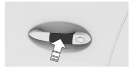
Hold the activated Key Card directly and centrally up against the outside door handle on the driver's door.
