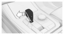
Press the selector lever out of selector lever position D to the left.
