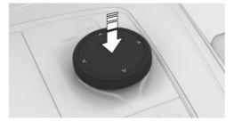
▷ Tilt in four directions to switch between screens, for example.
