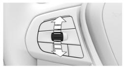
Press the rocker switch repeatedly up or down until the desired speed is set.
