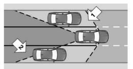
Operational from a minimum speed, radar sensors monitor the area behind and adjacent to the vehicle.
