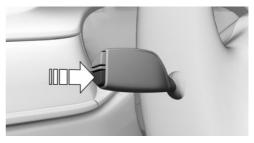
Press the button on the turn indicator lever.
