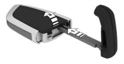
3. Use a pointed object to push the battery in the direction of the arrow and lift it out.
