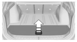
The first-aid kit is located in the compartment under the luggage compartment floor.
