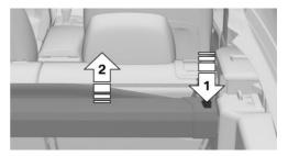
4. Remove the case upwards from both side brackets, arrow 2. Take care not to get the case jammed.
