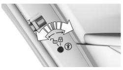
Unlock or lock the safety switches on the rear doors with the integrated key.
