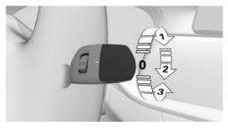
Turn the outer switch upwards.
