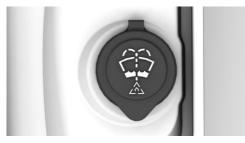
The reservoir for the washer fluid is located in the engine compartment.
