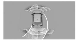
The vehicle's approach to an object is shown on the Control Display. Objects that are further away are already displayed before an acoustic signal is given.
