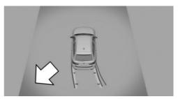
In the Park Distance Control PDC view, the relevant boundary area flashes red if the sensors detect vehicles.
