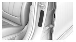
The tyre inflation pressure information is shown on the door pillar of the driver's door.
