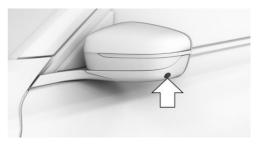
A camera is located under each exterior mirror housing.
