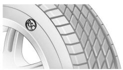
The tyres are identified by Runflat System Component RSC on the tyre's side wall.
