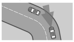
If the desired speed is too high for cornering, it will be reduced slightly in the bend. However, the system may not detect bends in advance, so moderate your speed when cornering.
