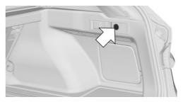
The button for swinging the swivel-mounted ball linkage in and out is in the luggage compartment.
