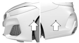
The Park Assist ultrasonic sensors are located on the side of the vehicle.
