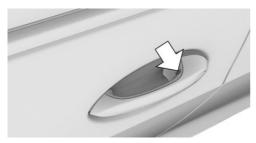
With your finger, touch the knurled area on the handle of a closed vehicle door and keep your finger there without gripping the door handle.
