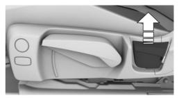
Pull the lever and apply your weight to or lift your weight off the backrest as required.
