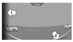
The relevant boundary area, arrow 1, in the camera view flashes red if the sensors detect vehicles.
