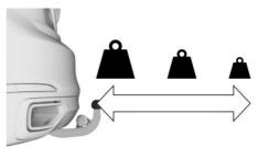
The permitted gross weight of the rear luggage rack when loaded depends on how far its centre of gravity is from the ball linkage.
