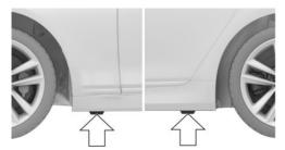
The jacking points are located in the marked positions.
