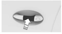
Hold the NFC antenna on the smartphone directly and centrally up against the outside door handle on the driver's door.
