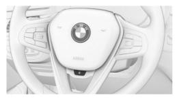
Button for steering wheel heating
