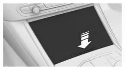
2. The ashtray is located in one of the cup holders. Fold the cover of the ashtray upwards.
