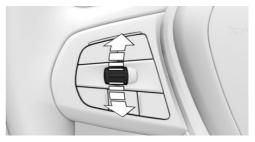
Press the rocker switch repeatedly up or down until the desired speed is set.
