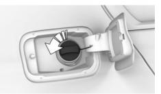
3. Place the fuel tank cap in the holder on the fuel filler flap.
