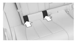
The fixtures for the lower ISOFIX anchors are located behind the marked covers.
