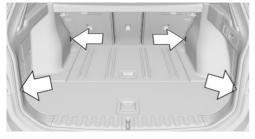
Four lashing eyes are located in the luggage compartment for securing loads.
