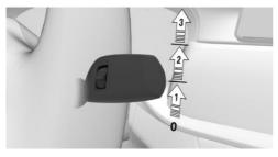
Press the lever upwards once from the home position, arrow 1.
