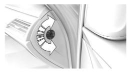
The key switch for front passenger airbags is located on the outside of the dashboard.
