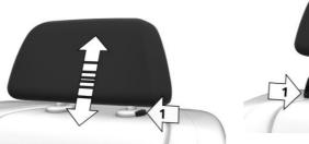
The outer head restraints can be adjusted in height.
