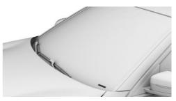
The vehicle identification number is additionally located behind the windscreen.
