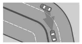
When your vehicle is approaching a bend, the angle of the bend may cause the system to respond temporarily to vehicles in the other lane. If the system responds by decelerating the vehicle, you may compensate for this by accelerating briefly. When the accelerator pedal is released again, the system will resume control of the vehicle's speed.
