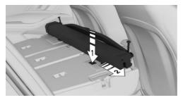
2. Push the case from above into both brackets in the side trim panel behind the rear seat
