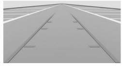
The driving path lines help you to estimate the space required when parking and manoeuvring on a level road surface.
