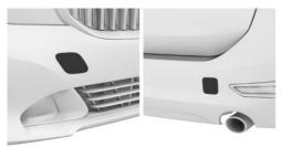
Press the marking on the edge of the cover to push it out.
