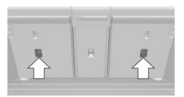
Depending on the equipment installed, there are two or three mounting points for the upper retaining strap of ISOFIX child restraint systems.
