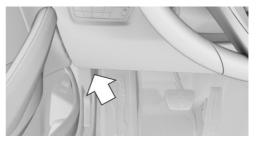
The OBD socket for checking emissions-relevant components is located on the driver's side.
