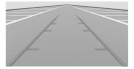
The driving path lines help you to estimate the space required when parking and manoeuvring on a level road surface.
