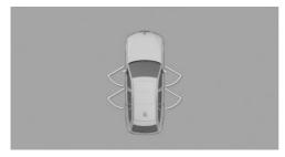
Steptronic transmission: the maximum door opening angles are displayed when the selector lever is in position P. Once the vehicle moves off, the parking assistance lines are displayed instead of the opening angles.
