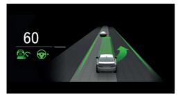
An example: the indicator and warning lamps for Active Cruise Control with Stop&Go function ACC and the lane change assistant indicate a move into the adjacent lane. At the same time, the move into the adjacent lane is shown as an animation in the Assisted Driving View.
