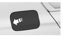
2. Turn the fuel tank cap anticlockwise.
