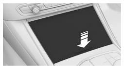
2. The socket is located between the cupholders. Pull off the cover.
