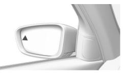
The light in the exterior mirror flashes if other vehicles are detected by the rear sensors when the vehicle is reversing.
