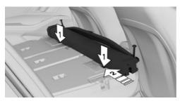
6. Push the case to the left until the guides reach their limit position, arrow 2. Make sure that the red mark on the backrest is no longer visible.
