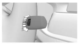
Turn the knurled wheel to set the sensitivity of the rain sensor.
