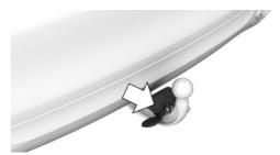
The trailer socket is located on the trailer tow hitch.
