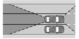
Four radar sensors in the bumpers monitor the area adjacent to the vehicle from a minimum speed up to approx. 210 km/h, 130 mph.
