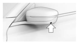
A camera is located under each exterior mirror housing.
