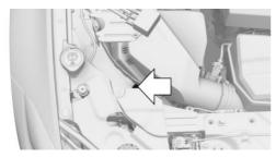
A special connection on the body serves as battery negative terminal.
