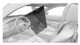
The camera in the roof lining detects gestures made in the area of the centre console at the height of the Control Display.
