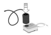
4. Screw the filler hose of the sealant container onto the tyre valve of the faulty wheel.
