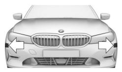
Depending on the equipment, there are two additional radar sensors in the front bumper.
