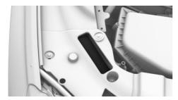
The vehicle identification number is in the engine compartment, on the right-hand side of the vehicle.
