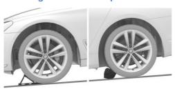
If it is necessary to change a wheel on a slight downhill slope, place chocks and other suitable objects, for example stones, under the wheels of the front and rear axles in the opposite direction to the direction of roll.
