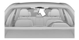
The camera is located near the rear-view mirror.
