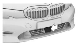
The radar sensor is located on the front in the bumper.
