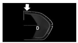
If the electric motor supports the internal combustion engine, for example in the case of heavy acceleration, eBOOST will be displayed. The level of eBOOST provided depends on the available charge state of the high-voltage battery. eBOOST might not be available at all if the charge state of the-voltage battery is low.
