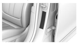
The tyre inflation pressures are shown on the door pillar of the driver's door.
