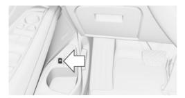
The button is located in the driver's door storage compartment.
