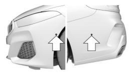
The system uses the four side ultrasonic sensors, arrows, and the ultrasonic sensors in the bumpers to measure parking spaces and distances to obstacles.
