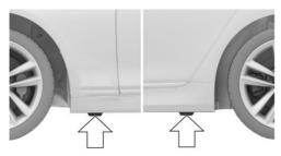
The jacking points are located in the marked positions.
