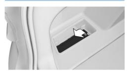
The on-board tool kit is located in the left storage compartment of the boot, under a cover.
