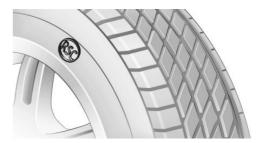
The tyres are identified on the tyre's side wall by RSC Runflat System Component.
