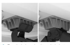
3. Turn the jack crank or lever clockwise to extend the jack.
