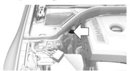
The jump-starting connection in the engine compartment serves as the positive battery terminal.
