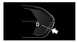
The energy recuperation when coasting and braking is displayed depending on the drive mode by the CHARGE display in the instrument cluster, see arrow. The high-voltage battery is charged. No energy can be recovered if highvoltage battery is fully charged.
