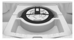
The emergency wheel and the wheel change tools are located in the boot under the floor.
