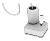
Let the compressor run for approximately 10 minutes to fill the sealing compound and achieve a tyre inflation pressure of approximately 2.0 bar.
