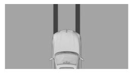
The washing bay view provides assistance when driving into washing bays by displaying the vehicle's own tyre tracks.
