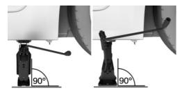
7. Raise by cranking until the jack is supported on the ground with its entire surface and the wheel in question is at most 3 cm, 1.2 inches off the around.
