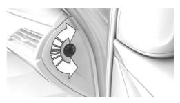
The key switch for front passenger airbags is located on the outside of the dashboard.
