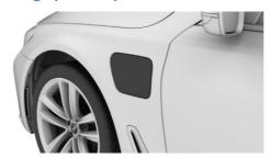
The charge point flap is located on the left of the vehicle.
