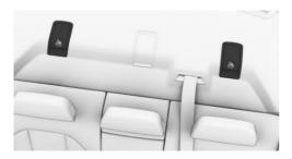
Depending on the equipment version, there are two or three mounting points for the upper retaining strap of ISOFIX child restraint systems.
