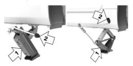
2. Guide the jack into the rectangular recess of the jacking point closest to the wheel to be changed.
