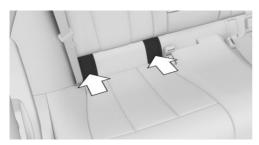
The brackets for the lower ISOFIX anchors are located behind the marked covers.
