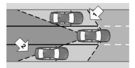
Operational from a minimum speed, two radar sensors in the rear bumper monitor the area behind and next to the vehicle.
