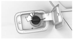
3. Place the fuel tank cap in the holder on the fuel filler flap.
