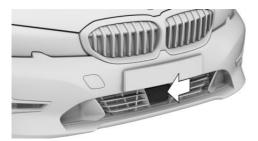
The radar sensor is in the lower area of the front bumper.
