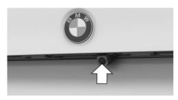
The camera lens is located in the handle strip of the boot lid.
